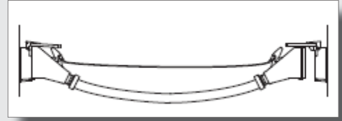
The locomotives move even farther apart. The resulting tension affects only the Safety Decoupler, allowing a safe and complete decoupling of the couplers. All coupler components remain intact.
